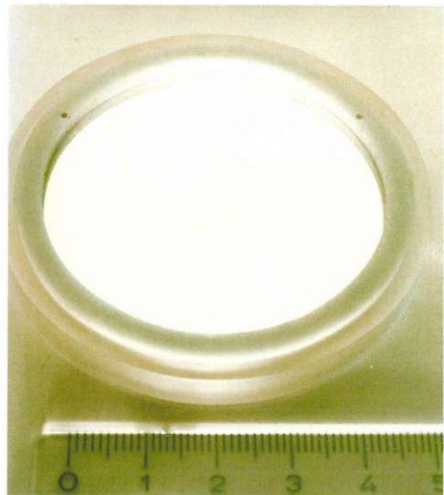
Fig. 14. Magnesium membrane 2 \mu\text{m} thick stretched over an aluminium-oxide ring.
