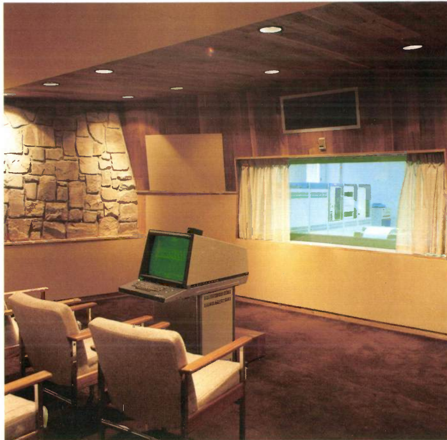
Fig. 1. Listening room and adjoining computer room. The listening room is well insulated against extraneous noise (background sound level 18 dB(A)). A computer terminal provides the listener with a direct control of the digital audio signal processing.
