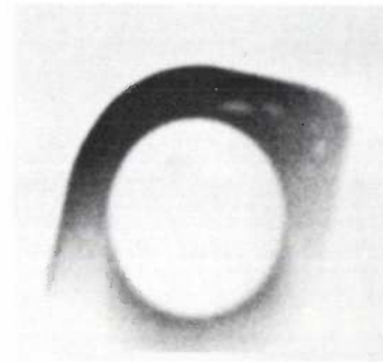
Fig. 4. A single-slice scatter image, again of the object Ob (fig. 1). This picture was made by means of a standard X-ray image intensifier connected to a television camera with a real-time video digitizer and a computer (for real-time processing of the video signal). Exposure time 0.64 seconds.
