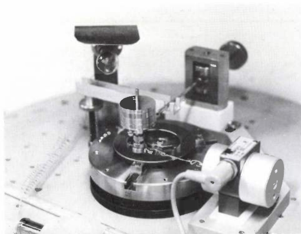
Fig. 4. Above: Diagram of the arrangement for friction measurements by the 'pin-on-disc' method. A substrate Sub with a diameter of about 75 mm, on which a film L has been deposited, rotates about a shaft A . Pressing on the substrate with a force F_1 (usually about 5 N) is a steel ball P of about 4 mm diameter, attached to a balance arm M . During the test a force F_2 acts on this pin; the force is measured by a force transducer. The coefficient of friction is defined as F_2/F_1 . Below: Photograph of a widely used experimental arrangement for friction and wear measurements.
