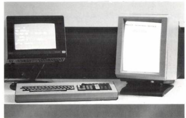
Fig. 6. The manager's terminal. This can be used to connect the user to the MEGADOC system and to show stored documents on a screen. The manager's terminal can be extended to include other functions such as electronic mail and access to data bases.
