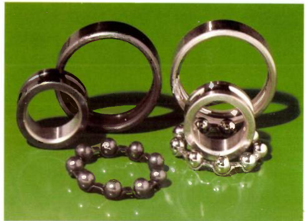
Fig. 18. Components of ball-bearings, coated with molybdenum sulphide (left) and uncoated.
