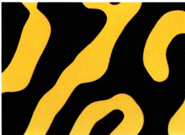
Fig. 17. Photomicrograph of the magnetic domains made visible when a 3- \mu\text{m} magneto-optical epitaxial film is illuminated by transmitted polarized light. The width of the domains is about 100 \mu\text{m} . The high contrast indicates a large Faraday rotation. This is achieved by bismuth substitution in the film.
