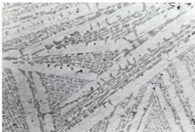
Fig. 1. Photomicrograph of a compound of La and Ni (57.2 at% Ni), taken after rapid cooling from the melt. The picture shows a polished and etched section. The many phase regions in the specimen are clearly visible. Magnification 200\times .
