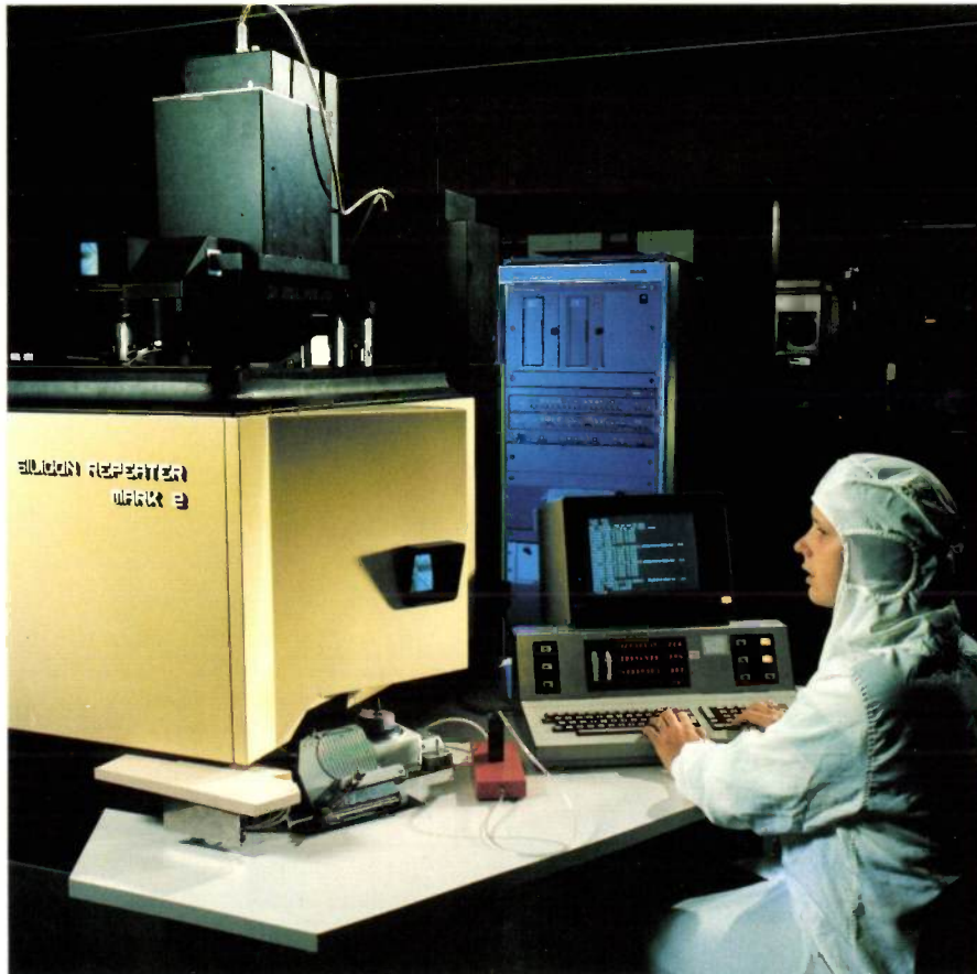
Fig. 1. The Mark 2 Silicon Repeater, an improved version of the earlier Silicon Repeater designed at Philips Research Laboratories and described in this journal [4]. The improved Silicon Repeater can expose sixty 4-inch silicon integrated-circuit wafers per hour.
