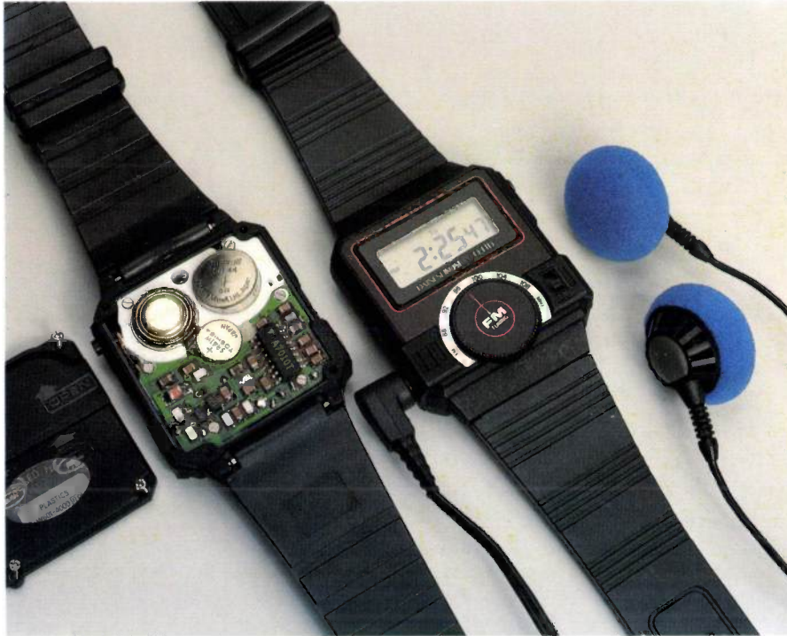
Fig. 3. A wrist-watch with a built-in FM receiver IC. The headphone lead also acts as the antenna.
