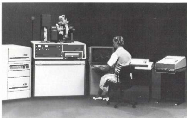
Fig. 5. The Philips PW 1700 Automated Powder Diffractometer System. The second cabinet from the left contains a high-voltage generator. Above it is an X-ray tube, which is connected to the diffractometer (on the right). The computer is at the far left, and on the right there are several output peripherals.
