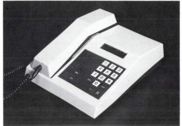
Fig. 5. The telephone adapted for DIVAC, with keys for abbreviated dialling, automatic redialling, and for cancelling an incorrect digit (R). It has a small screen for displaying a dialled number or a caller's number.
