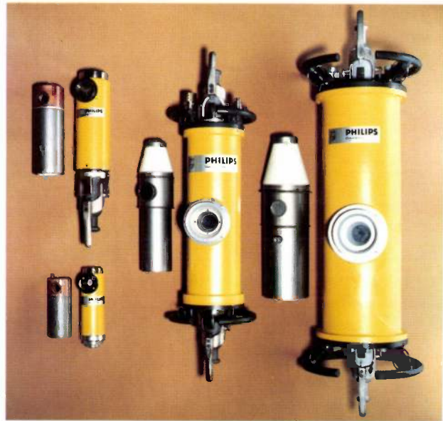
Fig. 4. The series of metal/ceramic X-ray tubes for macroscopic materials inspection. The tube alone and the tube with its shield are shown side by side. Left : two single-pole tubes for 100 kV maximum (below) and 160 kV. Centre : double-pole tube for 320 kV maximum. Right : double-pole tube for 420 kV maximum. The ceramic anode insulators can be seen in the double-pole tubes.
